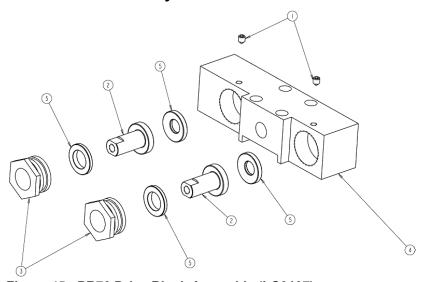
Figure 45: PR70 Drive Block Assembly (LC0107)
